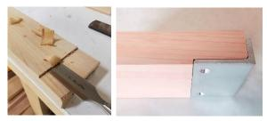
**NOTE**: Don't mortise a notch for the bracket under the bottom rail or skirt. The bracket is narrower than the wood and so close to the floor it will not be noticeable. And because the bracket is only slightly narrower than the wood, mortising the wood could cause the edges to split.
