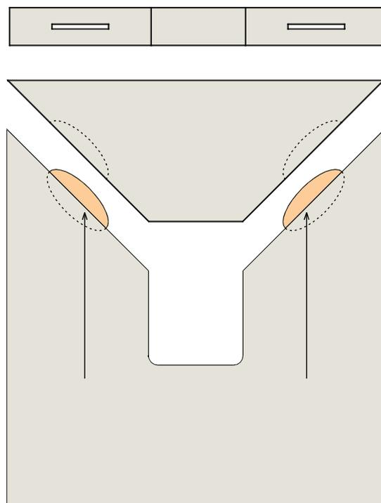
Plan view of "V" cut - shows jointer biscuit recessed into edge
