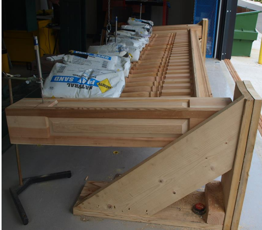
Figure 2: 6in rail at full load of 600lbs during the distributed load test
