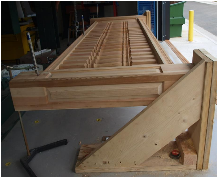
Figure 1: Set-up & fixture for rail testing
