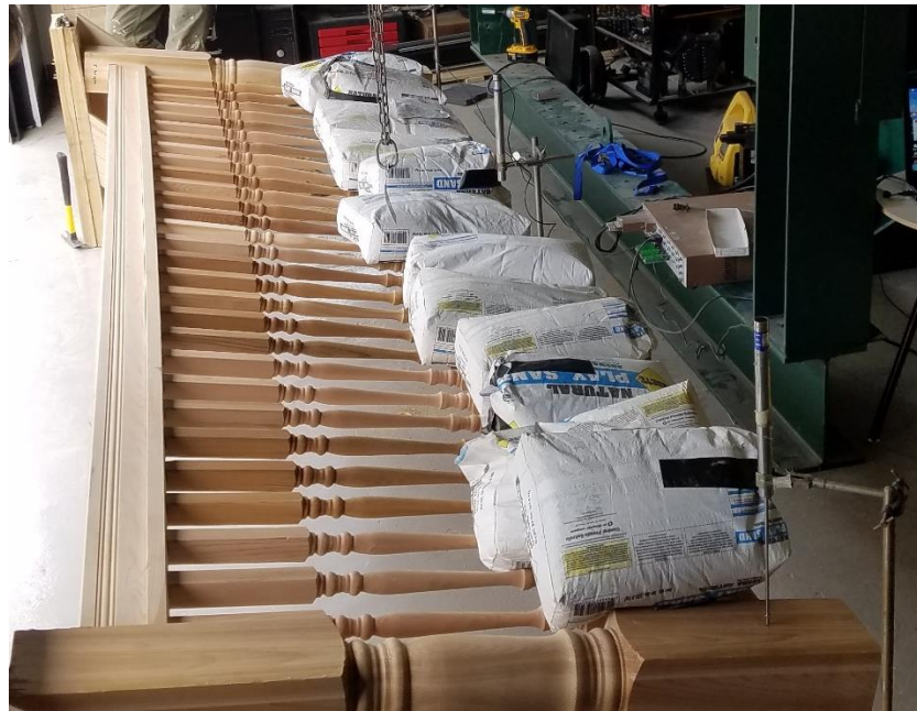
Figure 3: 4in rail at full load of 600lbs during the distributed load test
