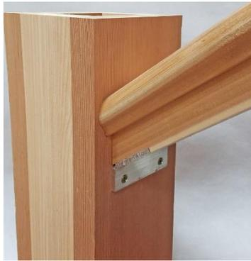
Mortise the post so that the shorter leg of the angle brackets are inset and flush with the surface of the newel post (with chisel or router).
