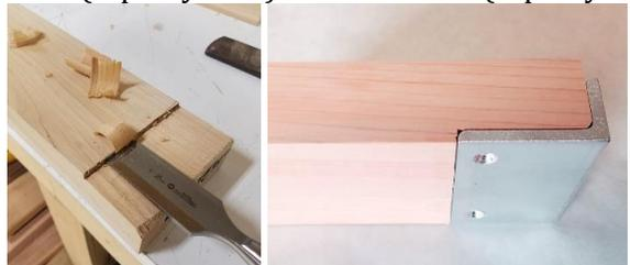
**NOTE:** with the 6" class 3-pc. System, you'll need to mortise a notch for the bracket to fit into the bottom rail because it is narrower than the rail. For the 4" class 3-pc. System, DO NOT mortise the underside of the bottom rail, because the bracket is only slightly narrower than the rail. A mortise on the 4" class Bottom Rail could cause the sides of the rail to split. The 4" class 3-pc. Bottom Rail simply sits on top of the bracket.
