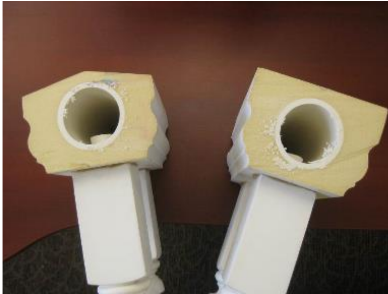
Photo No. 4 Top and Bottom Rail Profiles
