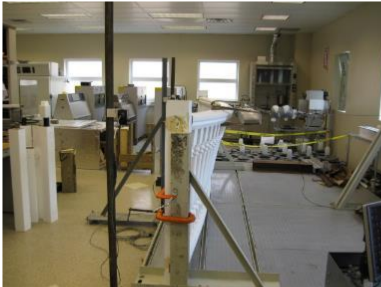
Photo No. 3 Horizontal Uniform Load Test of Top Rail
