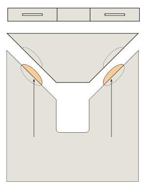
Plan view of "V" cut - shows jointer biscuit recessed into edge
