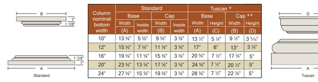
\* Tuscan cap/base have no platform—they wrap around the shaft. For inside widths, see the specifications for shaft inside widths. \*\* Tuscan cap widths may vary depending on height of shaft. The pitch (side angles) change and may require adjustment of cap width. Note: The total height of the parts (shown in the charts) do NOT add to the overall height of the column. The bottom and top plates do add 1" each (2" total) to the shaft height, allowing extra flexibility in installation.
